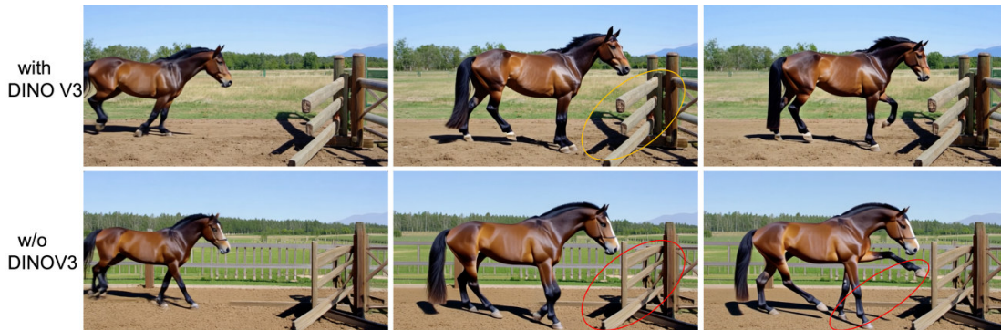
Figure 9. Effect of incorporating DINOv3 features. Adding DINOv3 supervision improves perceptual quality by preserving sharper details and more consistent object geometry. Without DINOv3, the generated content becomes overly smooth and may exhibit structural tearing around the horse and fence. Nevertheless, removing DINOv3 yields a higher Dynamic Degree and overall VBench score.
